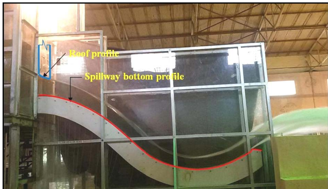
Fig. 5.2 Side view of physical model showing bottom and roof profile for experimental set up 3
